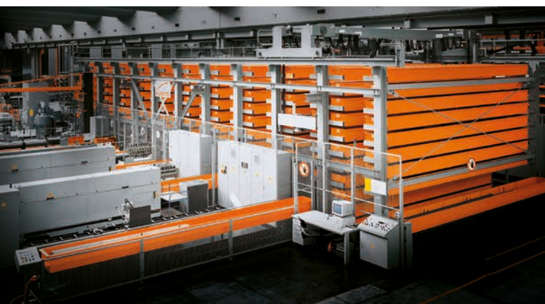
UNITOP : Bar storage system with a gantry crane moving on top. Due to fast access, also ideal as commissioning system.
