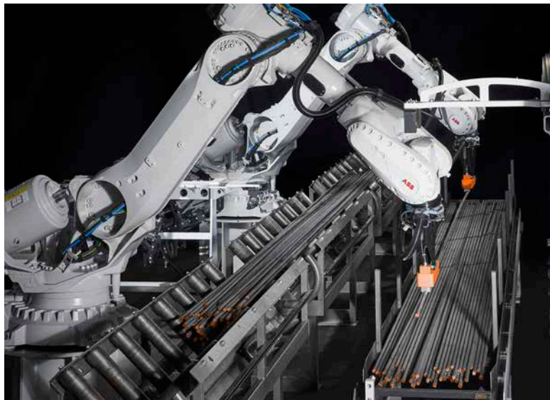
Bar removal with a magnetic gripper using KASTOpick bar
